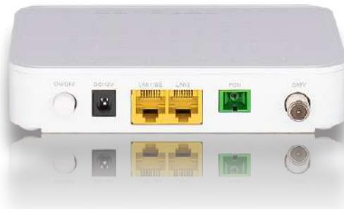
accurate bandwidth limit, which enables users to share 2.5Gbps (GPON) and 1.25Gbps (EPON) bandwidth resource appropriately. In addition, the QOS function of BDCOM GP1702-2FC-S guarantees a reliable service quality and service priority. It also supports QOS function, which guarantees a reliable service quality and service priority.
